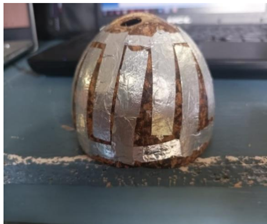
Figure 1. Side view of the coconut shells in the rain sensor
