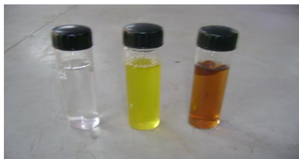
(a) 1 mM \text{AgNO}_3 solution (b) Leaf extract (c) Leaf extract + \text{AgNO}_3 after 48 h of reaction
