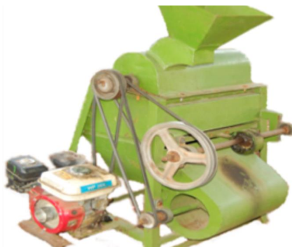
Fig 1. The coffee dehulling machine
